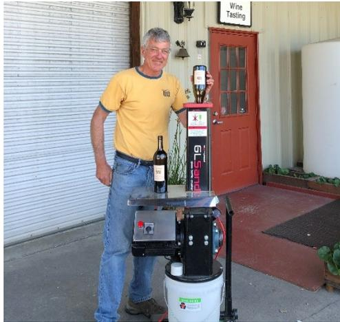
Chris with the new Glass Crusher! This machine has helped us divert over 100lbs of glass a week from landfill by turning bottles back into sand that is being used for landscaping projects.
